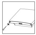
8 Install the upper door, fix the upper door hinge onto the cabinet.
