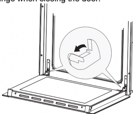
Tilting the hinge safety catches
