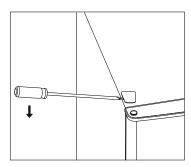
4. Move the core cover from left side to right side. And then lift the upper door and place it on a padded surface to prevent it from scratching.
