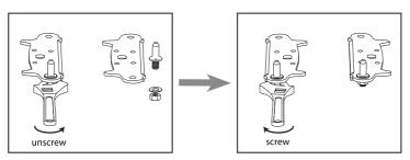
5. Refit the bracket fitting the bottom hinge pin. Replace both adjustable feet. Transfer the lower door to the property position.
