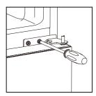
Laying down the refrigerator, take out the adjusting feet as below, then unscrew the lower hinge by cross screwdriver.
